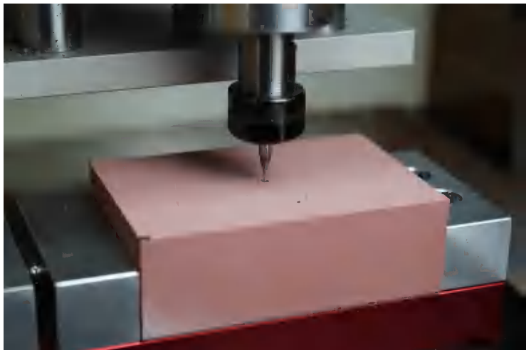
Figure 9-2. Origin at material center
