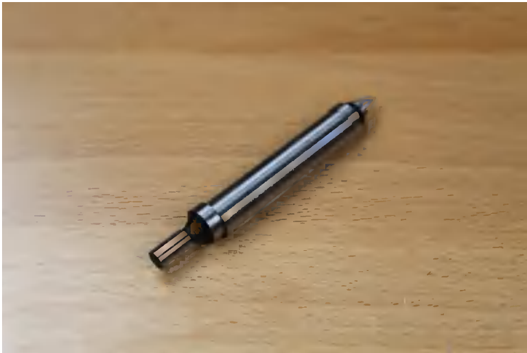
Figure 9-4. Basic edge finder with 1/4-inch shank
