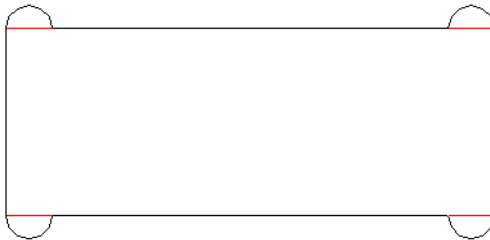
Figure 5-6. Overcutting with T-bones
