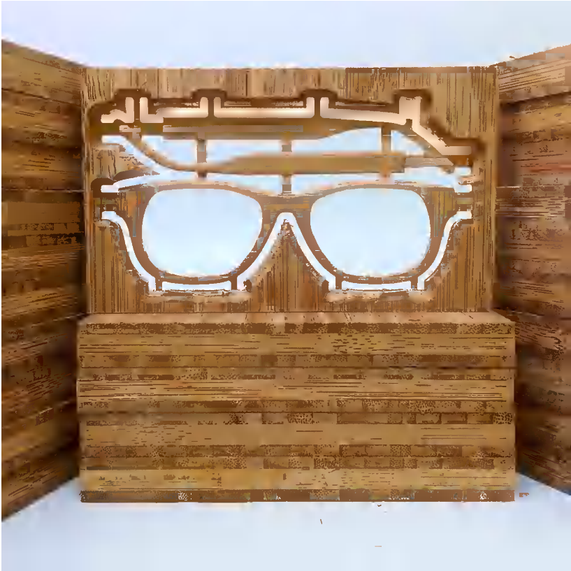
Figure 9-5. Holding tabs keeping finished sign secured to stock material
