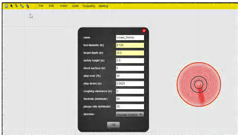
Figure 6-11. Pocket operation to reduce thickness of material
