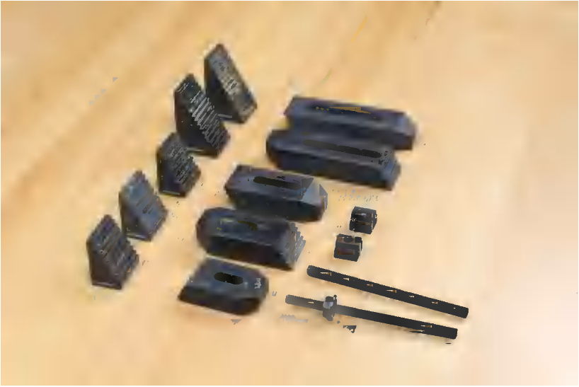
Figure 2-5. Parts of a step clamp
