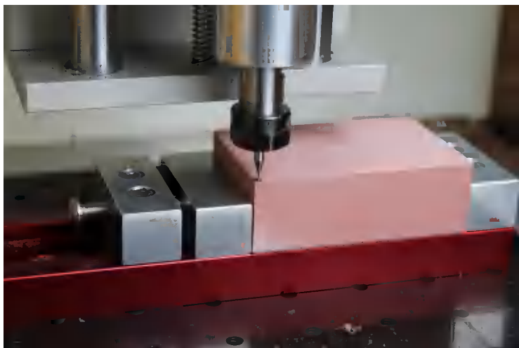
Figure 9-3. Origin at bottom-left corner
