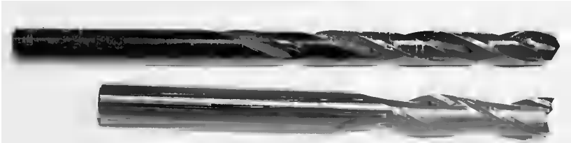
Figure 3-2. Comparison of a drill bit (top) and an end mill (bottom) —note the different tips
