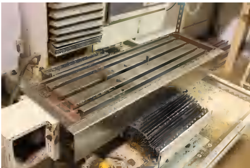
Figure 2-7. T-slots shown with T-nut and screw protruding upward from a Tormach PCNC 1100
